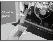
Open the lid on the top of generator, unscrew the oil cap then fill the oil until reaching the limit of the oil gauge. Finally, screw back the cylinder head stud.
