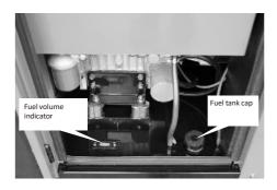
Open the left door, check the fuel volume indicator. If the fuel level is low, unscrew the tank cap, fill the fuel through the fuel filter. After filling fuel, screw back the tank cap.
