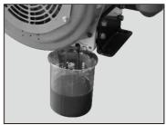
Open the lock over the front cover, screw the oil cap off as shown in the photo, pour the oil until reaching the limit of the oil gauge. Finally, screw back the cylinder head stud.
