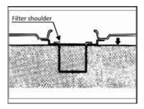
Overfilling is dangerous. Do not fill the tank beyond the top of the fuel filter shoulder.
